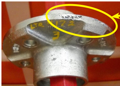
Sample of GAL-DEX Hub after 500 Hours of Salt Spray
