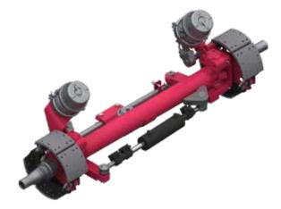
You can now add a heavy duty off-the-shelf, double acting hydraulic cylinder to your inline king pin package. It is rated for 3,000 psi and comes with industry standard tie-rod ends, which are common with tie-rods on the basic inline kin pin axle. It has a customizable push rod length to handle any axle track you require. Get the full package and simplify your installation when you choose Dexter's fully integrated ISS suspension system.
