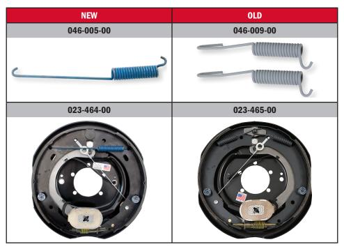
When performing service, be sure to identify which version of brake you have. The pictures below highlight the different anchor posts used on both the single and dual retractor spring designs. Like components should always be replaced with like components, as using different component combinations can cause brake performance issues or potentially cause the brake to malfunction.
