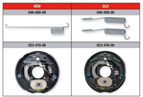
When performing service, be sure to identify which version of brake you have. The pictures below highlight the different anchor posts used on both the single and dual retractor spring designs. Like components should always be replaced with like components, as using different component combinations can cause brake performance issues or potentially cause the brake to malfunction.
