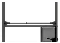
5. When mounts are seated into frame (shown), use one self-drilling screw per side (3 included) to fix the bar to the door frame. This requires a power drill/driver. Do not overtighten!
