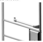
4. When mounts are nested into the frame sides, slide the assembly down until it touches the crossbar as shown.
