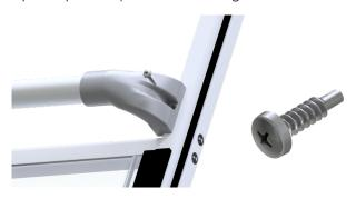
6. When the mounting screws are in place, make sure the center bushing is firmly pushed into the large tube. Use the third screw and install into the hole shown using the drill driver. This will fix the bushing/tubes/assembly firmly.
