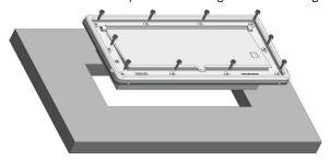
4. Install cover by sliding down onto flange aligning the (3) locking tabs in the cover and the (3) receiving slots in the flange.
