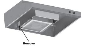
2. Remove 'C' clamp from slide lever and set aside for later installation. Place slide lever into slot on blower housing as shown.
