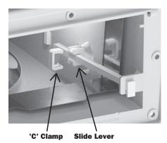
8. Move slide lever and slide rod assembly to the full open position.
