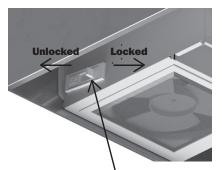
Slide lever toward wall to unlock and opposite to lock damper
