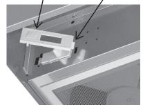
4. Remove wall vent cover (not shown) and damper. Remove square knockout in lower right hand corner of damper; set damper aside for later installation.
