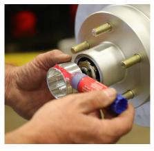
12. Then install it onto the hub using a hammer with a block of wood or a mallet. Apply firm straight blows until the aluminum housing is fully seated. Wipe off any excess red sealant.
