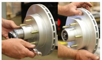
5. Remove the seal and inner bearing from the hub assembly.
