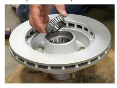
8. Lightly lubricate the outer diameter of the seal, then seat it into the hub. Lubricate the inner diameter of the seal, ensuring the seal is fully seated.
