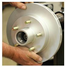
11. Ensure the opening of the hub is clean. Apply a small bead of red sealant on the cap's aluminum housing mating surface.
