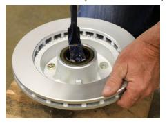
6. Clean bearings and hub thoroughly with a degreaser to ensure no old lubrication exists. If there are signs of corrosion or wear, replace the affected parts before continuing the installation.
