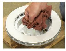
7. Install inner bearing into hub assembly.
