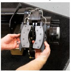
4. Align the brake pad mounting holes with the holes in the caliper. Insert two (2) brake pad retaining pins into each caliper half. Place the anti-rattle spring against the brake pads and press the center toward the rotor while you slide the outboard pad retaining pin toward the inner lining. Continue sliding the pad retainer pin until it engages both pads and pushes the second pin out of the inboard caliper half.
