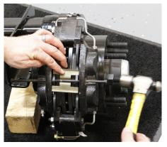
5. Install the locknut snug to the retaining bolt, do not exceed 4 Ft. Lbs. of torque, or install the cotter through the hole in the retaining pin.
