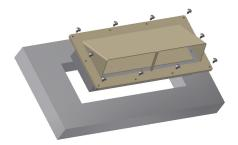
4. Apply sealant of choice in seams of the wall, cover top and sides. Note: damper lock is shown in the open position, to lock damper push up past the detent.
