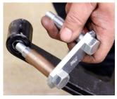
insert the punch (or bolt) into the bushing and drive it into place by firmly striking the punch (or bolt) with a suitable hammer.
