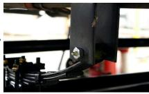
approximately 3/8" inside diameter to encircle the grease fitting in the head of the bolt. Strike the end of the tube squarely and firmly. Avoid glancing blows.
