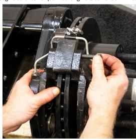
4. For brakes produced after April 2008, apply anti-seize or similar thread lubricant to the 1/4-20 bolt and reattach the crossover line tube clamp to the inboard side of the yoke. Torque the bolt to 85-100 lnch Lbs.
