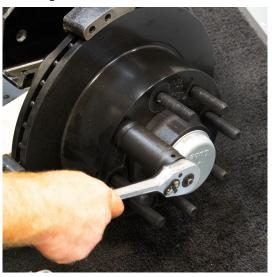
Remount the caliper assembly onto the caliper attaching bracket.
