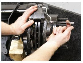
6. For brakes produced after April 2008, the crossover brake line also attaches to the inboard side of the caliper mounting bracket using the metal tube clamp. Slide the clamp over the crossover brake line and bend it to the closed position. Apply anti-seize or similar thread lubricant to the 1/4-20, 1/2" length bolt. Attach the tube clamp to the threaded hole in the caliper mounting bracket using the 1/4-20, 1/2" length bolt. Torque to **85-100 Inch Lbs.**
