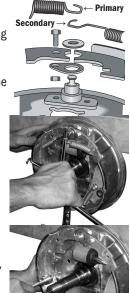
backing brakes, remove the bolt, lock nut, and retaining loop from the top of the primary shoe and the pivoting pin, spring, bolt, and nut from the bottom of the shoe. Retain them for later re-installation on the replacement shoes.
