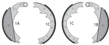
IT IS RECOMMENDED THAT ALL FOUR (4) SHOE/LININGS BE REPLACED AT THE SAME TIME TO ENSURE BALANCED BRAKING PERFORMANCE. The brakes and shoes shown above are free backing with pivoting primary brake shoes. If your kit is for standard style brakes, both shoes will look similar with the primary shoes having the shortest length brake linings. Primary shoes should be installed to face the front of the trailer, while the secondary shoes face the rear of the trailer.
