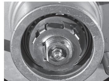
5. If the nut is too tight, remove the retainer and back the nut off approximately one twelfth of a turn and reinstall the retainer. The nut should now be free to move slightly.
