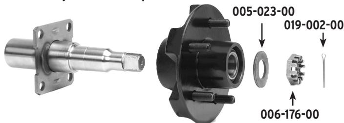
2. Leave the hub or hub-drum stationary and slowly loosen the wrench just until the torque on the nut goes to zero. **NOTE: THE TORQUE WILL TYPICALLY GO TO ZERO - DO NOT CONTINUE TO LOOSEN.**
